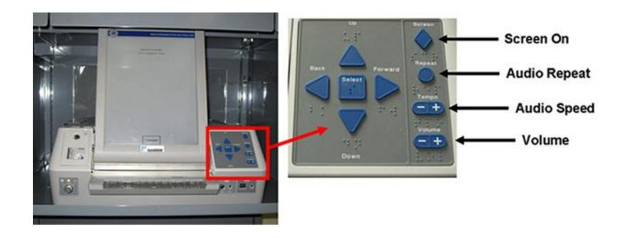
Navigating the AutoMARK to mark a ballot using the keyboard
