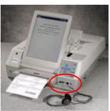
Headphones would get plugged into the front of the machine as shown
